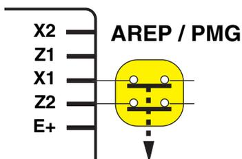
The exciter is switched off by disconnecting the AVR power supply (1 wire on each auxiliary winding) - contact rating 16 A - 250 V AC. Connection is identical for resetting the AVR internal protection.
