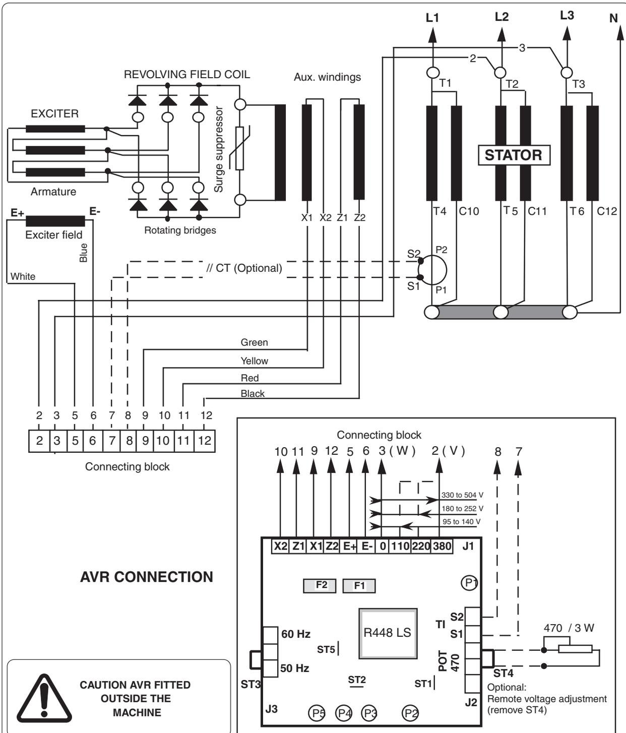
WIRING AND AVR CONNECTION DIAGRAM
