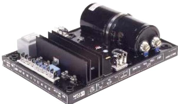
With **AREP** excitation, the R 448 electronic AVR is powered by two auxiliary windings which are independent of the voltage match circuit. The first winding has a voltage in proportion to that of the alternator (characteristic Shunt), the second has a voltage in proportion to the stator current (compound characteristic: Booster effect). The power supply voltage is rectified and filtered before being used by the AVR monitoring transistor.
