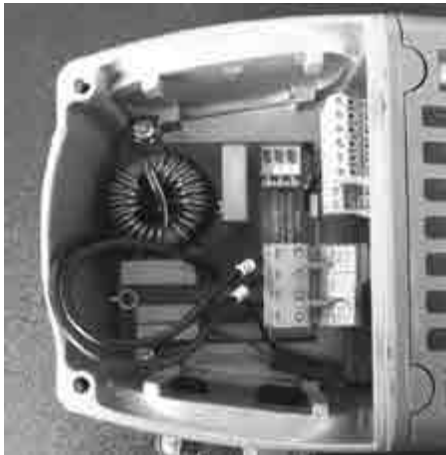
Internal filter FLT VMA31M/32M 110 for single phase range
