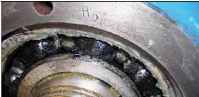
Illustration 7 - Bearing grease blackened following overheating due to multiple discharges
