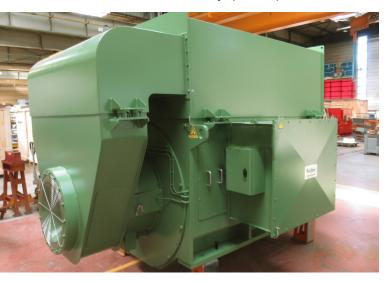
After detailed deliberation all parties, we finalized the design. Once built, the alternator was subjected to the Factory Acceptance Test at the Nidec Leroy-Somer works in France, on a unique special test platform, where it is subjected to a closed loop test at full load.
