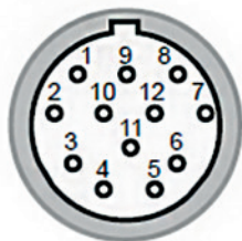
View of M23 female connector base (Counter clockwise) user side
