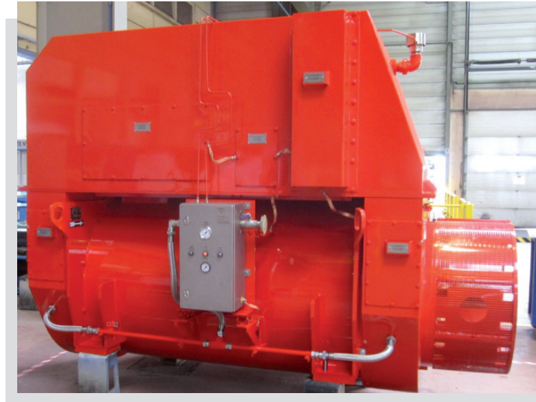
Pressurised Hydro-refrigerated machine for use in offshore oil exploitation in a hazardous environment
