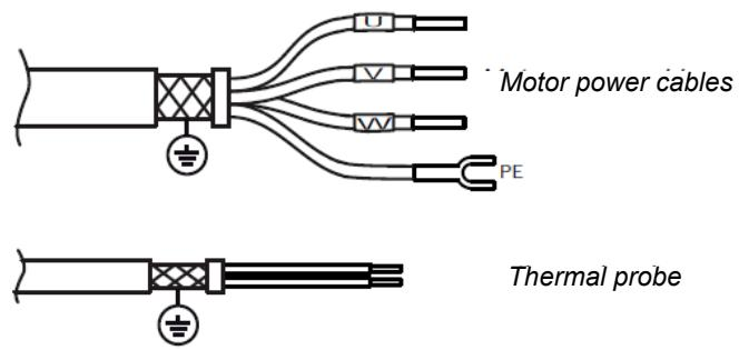
Connect the motor by using cables of the correct cross-section (the cables and terminals must be sized according to the current, see table below).
