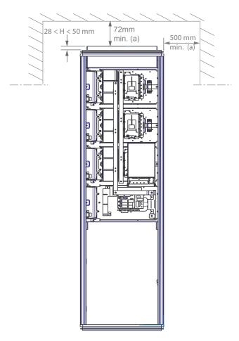
(a): Distance between the roof of the cabinet and an obstacle (e.g. wall, etc). Several cabinets can be assembled together (ensure that the air is extracted correctly).
