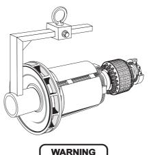
When dismantling the rotor involves changing parts or rewinding, the rotor must be rebalanced.
