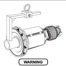
When dismantling the rotor involves changing parts or rewinding, the rotor must be rebalanced.
