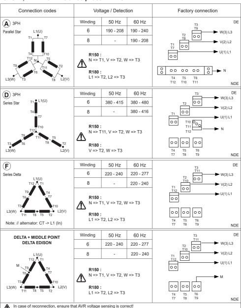
The factory can supply a set of flexible shunts and special connection links as an option for making these connections.
