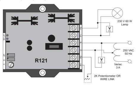
This test should only be attempted after making sure that the AVR has passed all multimeter checks. Connect the AVR to the single-phase variable voltage source as shown in diagram 1 in this manual.
