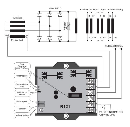
The AVR builds up the generator voltage from its residual voltage to rated voltage.
