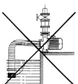
If the pump is working on load, the bottom valve is replaced by an isolation valve on the pump.
