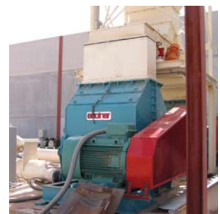
The entire wood waste energy conversion process at the Villacañas biomass factory is equipped with LS motors, geared motors and an alternator, all certified to operate in explosive atmospheres (ATEX dust).
