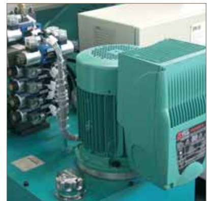
Hydraulic unit intended for driving sheet metal transformation machines (long-table bending presses) fitted with a motor with integrated frequency inverter, of the Leroy-Somer Varmeca type. All functions, acceleration, braking and the various speed movements are controlled by the Varmeca frequency inverter mounted on the pump motor.
