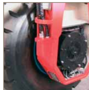
HPM motor integrated in the wheel hub
