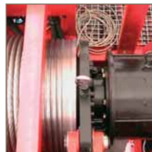
HPM motor integrated in the winch drum
