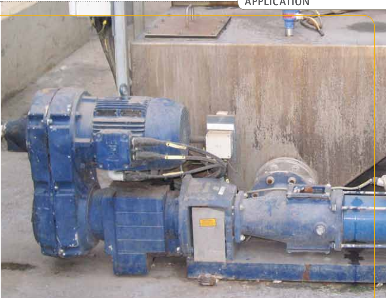
The old system containing a belt variator was liable to breakdowns.
