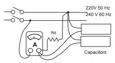
Rd: discharging resistor (5000  $\Omega$  - 20W) The currents are indicated at ± 10%
