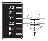
The exciter is switched off by disconnecting the AVR power supply (1 wire on each auxiliary winding) - contact rating 16 A -250V A.C.
