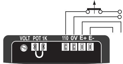
The exciter is switched off by disconnecting the AVR power supply.
