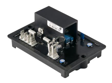
R220 is an analog AVR with power controlled by transistors. It is designed for small alternators with a SHUNT excitation.
