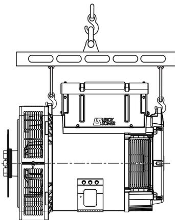
The TAL 044 is equipped with two air deflectors that prevent access to the upper and lower holes of the flange. Coupling for this machine should be done with screws in the eight accessible holes, disregarding the ones that cannot be accessed because of the deflectors.
