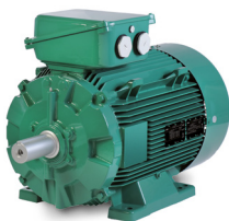
LS / LSES Non IE- IE2- IE3 Aluminium IP55 Frame size 56 to 315 mm 2, 4, 6 and 8 poles 0.09 to 200 kW
