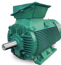
FLSES IE3 - IE4 IP55 cast iron Frame size 80 to 450 mm 2, 4, 6 and 8 poles 0.75 to 900 kW
