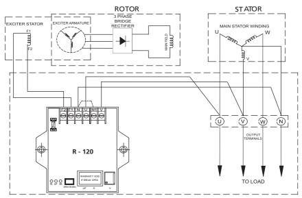
Note : For 1 Phase connection connect, between U & N Put short link between N & N1
