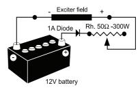
**Assembly B**: Connect a "Variac" variable power supply and diode bridge on both exciter field wires (+) and (-). Both these systems should have characteristics which are compatible with the machine field excitation power (see the nameplate).
