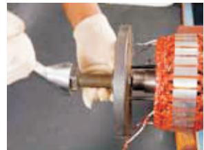
EXCITER ROTOR REMOVAL
