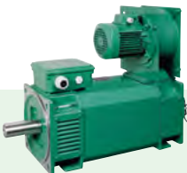
CPLS Aluminium IP23 Frame size 132 up to 250 mm 7.5 up to 560 kW Speed up to 6,000 rpm
