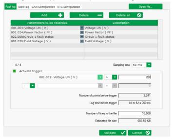
The "Fast Log" tab allows to select up to 4 parameters for logging with short sampling time down to 50ms whilst "Slow log" tab allows up to 6 parameters with minimum sampling time of 1 minute.
