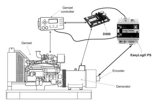
Encoder information is transmitted to the D550 by the EasyLogPS to be processed.
