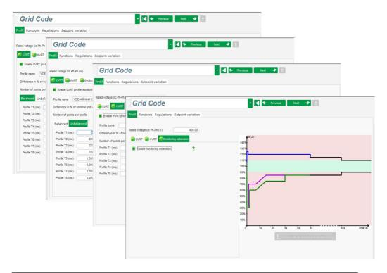
Enabling Voltage monitoring will activate an alarm/digital output when the measured voltage will cross the profile and therefore is out of the FRT profile.
