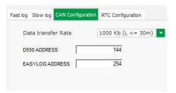
On this figure, the data transfer rate, the D550 address and EasyLog/EasyLogPS are to be configured with the same values as those defined on the D550 otherwise the communication will fail
