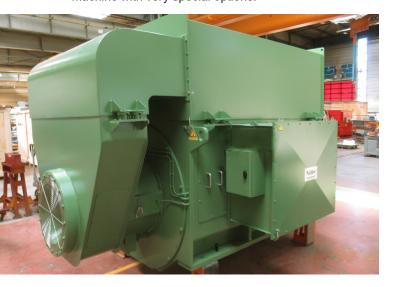
After detailed deliberation all parties, we finalized the design. Once built, the alternator was subjected to the Factory Acceptance Test at the Nidec Power works in France, on a unique special test platform, where it is subjected to a closed loop test at full load.
