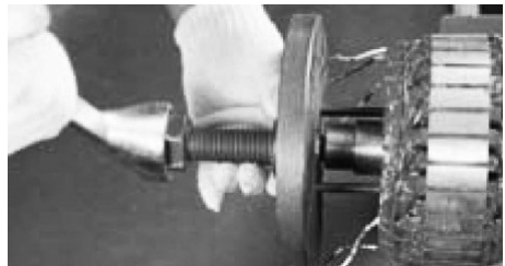
Exciter rotor removal
