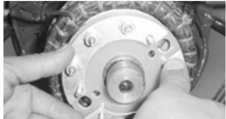
Rotating rectifier assembly removal
