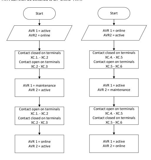
Note: The "active" AVR cannot be set to "maintenance" mode if regulation is occurring and the second AVR is in "maintenance" or "fault" mode.
