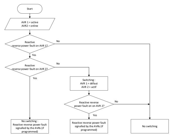
Note: By default, no action has been programmed for reactive reverse power. A significant bump may therefore occur on switching to the "online" AVR. This bump may be less noticeable if the "field current before fault" action has been selected.
