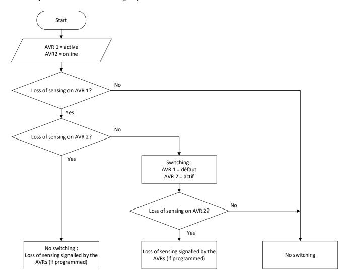
Note: By default, no action has been programmed for loss of sensing. A significant bump may therefore occur on switching to the "online" AVR. This bump may be less noticeable if the "field current before fault" action has been selected.
