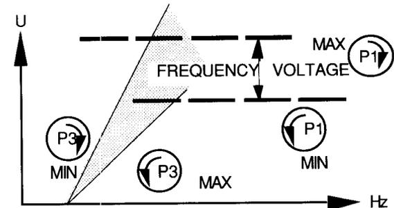
Potentiometer (P1) MAXIMUM voltage fully clockwise
