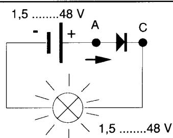
A diode in a good condition enables the current to flow in only one direction from anode to cathode.
