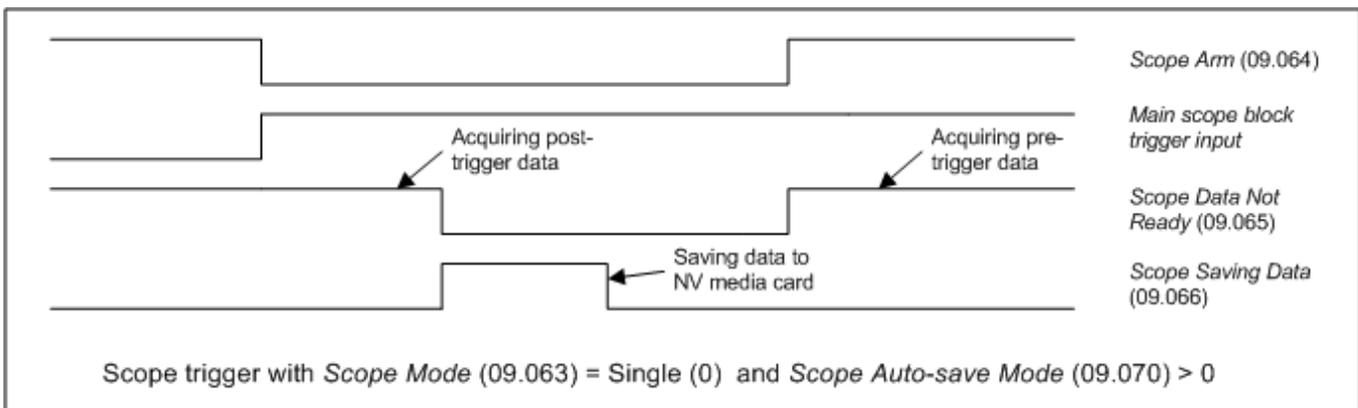
It is possible to read scope files via comms or into an option module. However, scope file transfer can only be initiated when *Scope Arm* (09.064) = 0, *Scope Data Not Ready* (09.065) = 0, *Scope Saving Data* (09.066) = 0 and at least one trace has been set up. While the file transfer is in progress *Scope Saving Data* (09.066) is set to 1.
