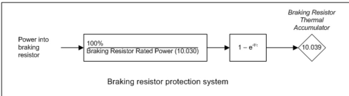
The drive monitors the power flowing into the braking resistor and updates the *Braking Resistor Thermal Accumulator* (10.039). If bit 1 of *Action On Trip Detection* (10.037) = 0 and the accumulator reaches 100% an *Brake R Too Hot* trip is initiated. If bit 1 of *Action On Trip Detection* (10.037) = 1 and the accumulator reaches 100% the braking IGBT is disabled until the accumulator falls below 95.0%.
