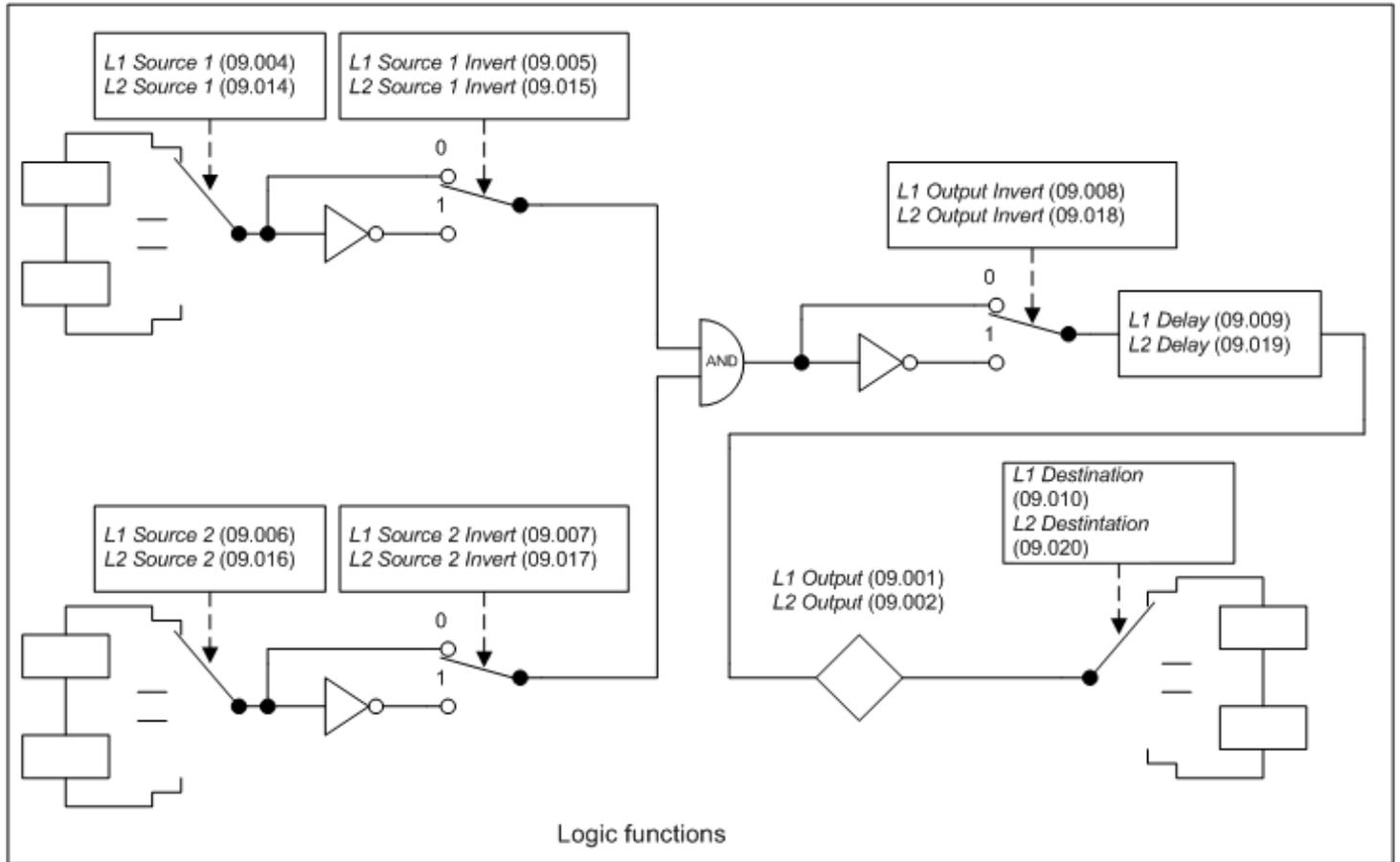
The logic function consists of an AND gate with inverters on each input and an inverter on the output. Some of the other standard logic functions can be produced as shown in the table below.
