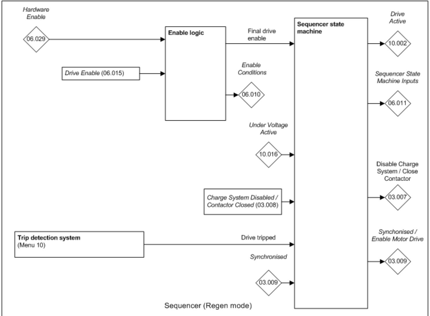
The sequencer, which provides overall control of the drive, is implemented in two stages. The first stage include the enable logic and consists of static logic elements. The second stage is a state machine with internal states.
