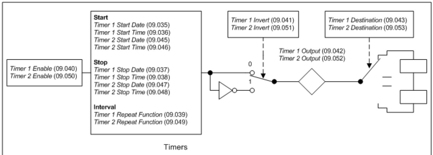
The following is a description of Timer 1, but Timer 2 behaves in the same way. If *Timer 1 Invert* (09.041) = 0 then *Timer 1 Output* (09.042) is inactive before the *Timer 1 Start Date* (09.035) / *Timer 1 Start Time* (09.036), active between this date/time and *Timer 1 Stop Date* (09.037) / *Timer 1 Stop Time* (09.038) and then inactive after the stop time/date within the timer 1 repeat period as shown in the diagram below.
