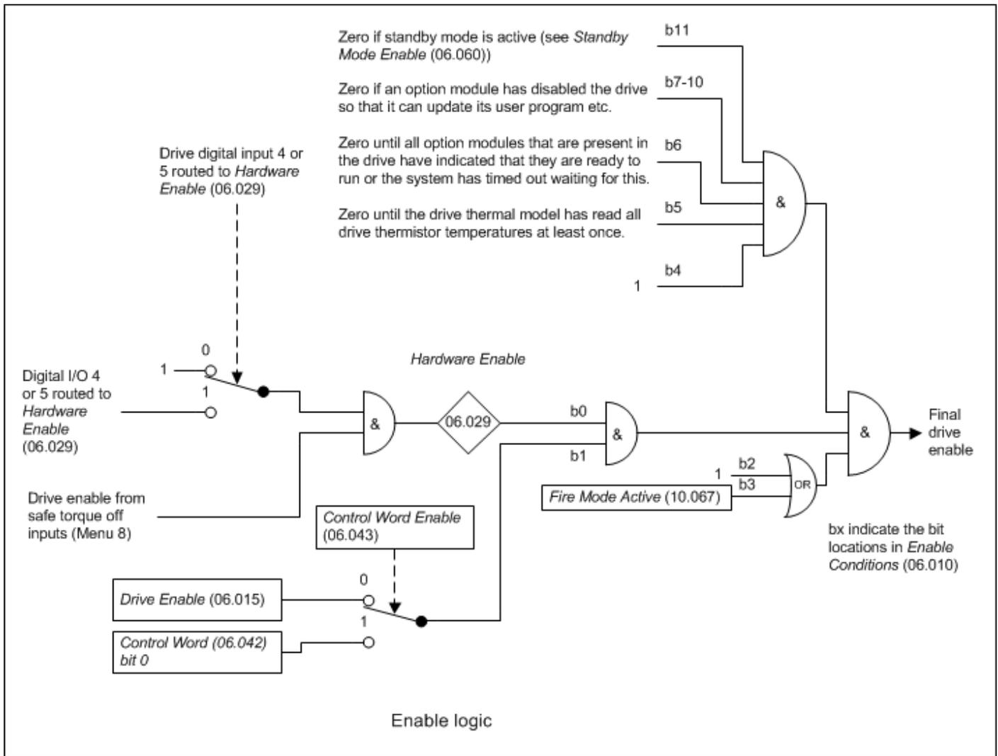
*Hardware Enable* (06.029) follows the safe torque off enable signal provided none of the digital inputs that are integral to the drive are routed to the *Hardware Enable* (06.029). The safe torque off hardware includes a delay in detecting a change from the enable to disable state of up to 20ms, but for most applications this is not a problem. However, a faster disable time can be achieved (600us) if digital input 4 or 5 on the drive is routed to the *Hardware Enable* (06.029).
