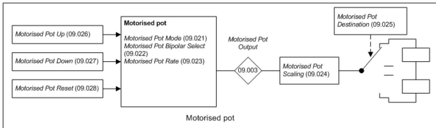
If *Motorised Pot Reset* (09.028) = 1 then the motorised pot is disabled and held in its reset state with *Motorised Pot Output* (09.003) = 0.0%. If *Motorised Pot Reset* (09.028) = 0 the motorised pot is enabled even if *Motorised Pot Destination* (09.025) is not routed to a valid parameter. The sample rate of the motorised pot is always 4ms.
