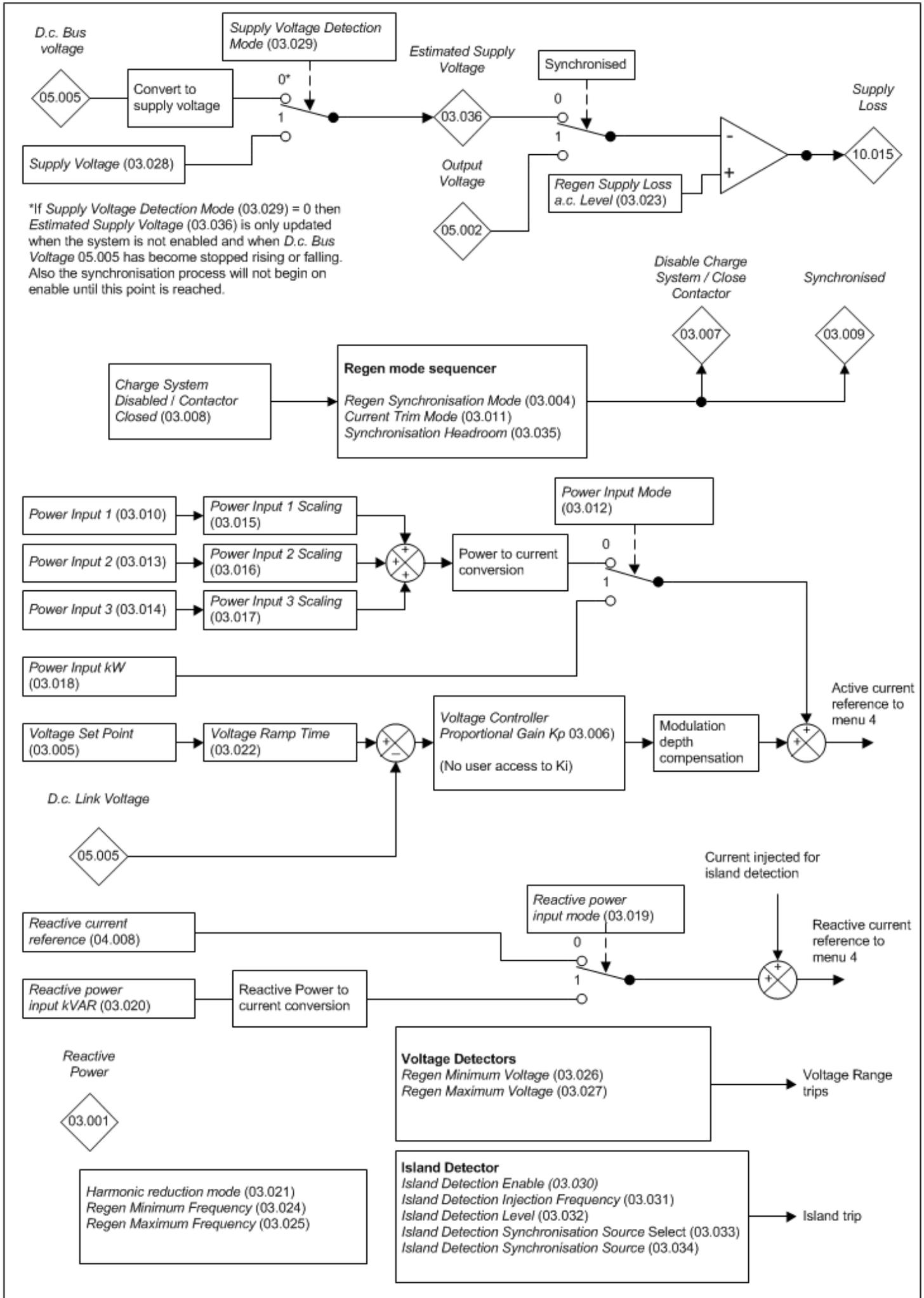
\*If Supply Voltage Detection Mode (03.029) = 0 then Estimated Supply Voltage (03.036) is only updated when the system is not enabled and when D.c. Bus Voltage 05.005 has become stopped rising or falling. Also the synchronisation process will not begin on enable until this point is reached.
