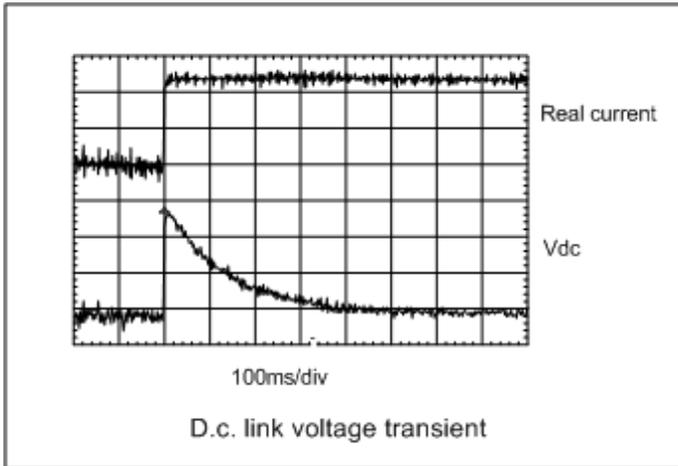
The example shown is for a very rapid load change where the torque reference of the motor drive has been changed instantly from one value to another. The peak of the resulting transient is
