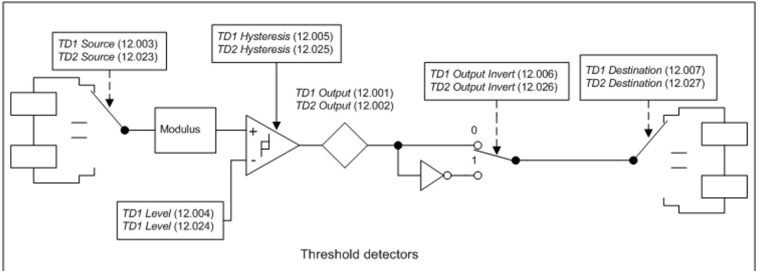
The following description is for threshold detector 1, but threshold detector 2 operates in the same way. The level of the parameter defined by *Threshold Detector 1 Source* (12.003) is converted to a percentage and compared to *Threshold Detector 1 Level* (12.004) with hysteresis to give *Threshold Detector 1 Output* (12.001) as follows:
