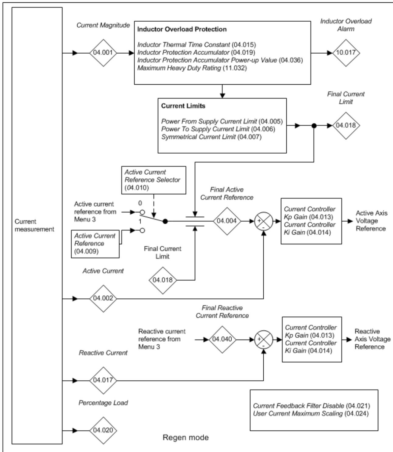
In Regen mode separate current control is provided for the active and reactive currents. The active current reference is normally produced by the d.c. bus voltage controller and power feed-forwards system, although it is possible for the user to define the active current reference if required. The reactive current reference is either defined directly from the *Reactive Current Reference* (04.008) or from the *Reactive Power Input kVAR* (03.020). See Menu 3 for more details.
