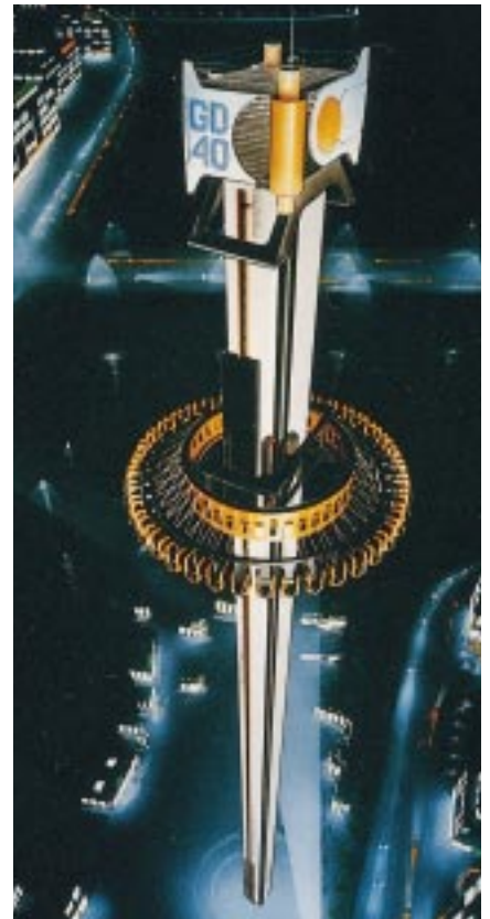
GYRO DROP. Using two DC motors LSK 2804 CL - 450 kW
