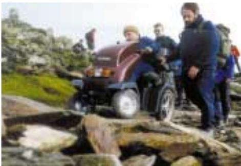
Motive power for the Tramper is supplied by a high performance, Leroy Somer CbZ, 24 V DC motor. Its outstanding 95% efficiency and ability to withstand the rough service inherent in this unusual application, makes it an ideal choice.
