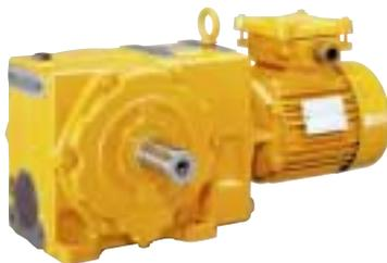
The new ranges of geared motors can be supplied with LSPX/FLSPX motors with or without brake and were developed to operate in dusty atmospheres where storage and handling of organic materials can produce flammable dust (cereals, greases, foodstuffs). The range starts at 0.09 and is completed by the 400 KW. The product fully conforms to the requirements of ATEX 94/9/CE, where the characteristics and the surface temperature of 125°C are guaranteed and a sealing protection to dust of IP65.
