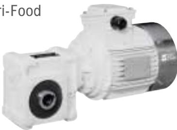
The main challenge for geared motors, in this market sector, is corrosion. The new range of worm and wheel reducers, the Multibloc 2000 IA and the CB 3000, incorporate many remarkable improvements: water retention zones reduced, reinforcement of mechanical seals and electrical connections, elimination of fretting corrosion.
